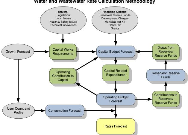
Figure 1-1 Water and Wastewater Rate Calculation Methodology
