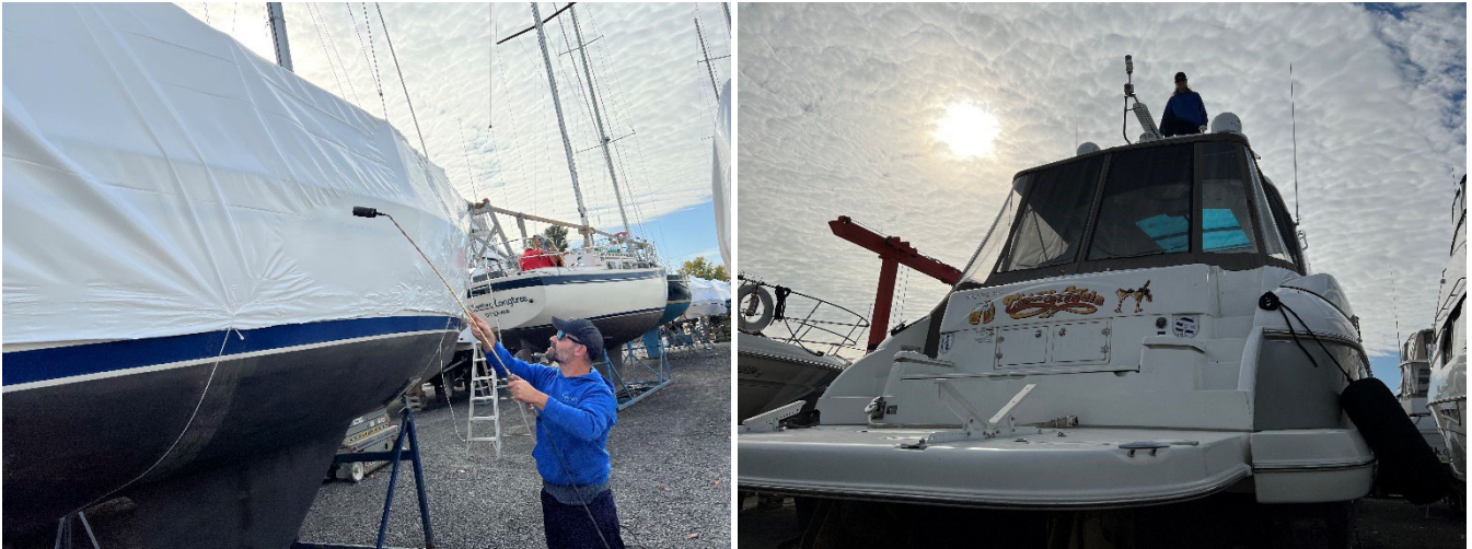
Figure 8: Process of heating shrink wrap using propane (left) and taller required working heights (right) (Source: Peck’s Marina)
